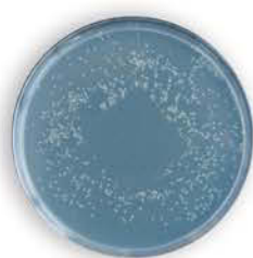
Petri dish containing a film with antimicrobial BactiBlock®. Inhibited bacterial ( E. coli ) growth on the film.
